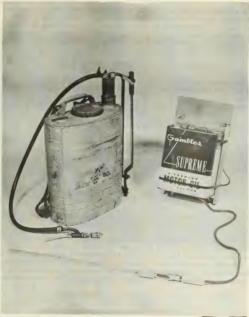
Figure 12.--Equipment used in high release by means of cut-surface treatment with 2,4,5-T. Knapsack sprayer which builds up pressure by means of pump operated with the right hand (on left); homemade gravity herbicide applicator (on right).
